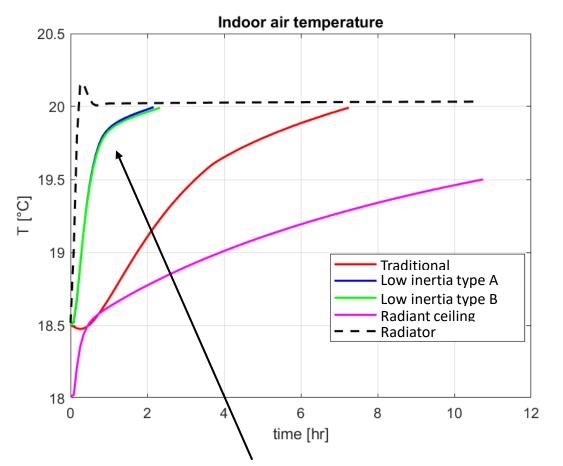
Very fast response for low-inertia radiant floor
