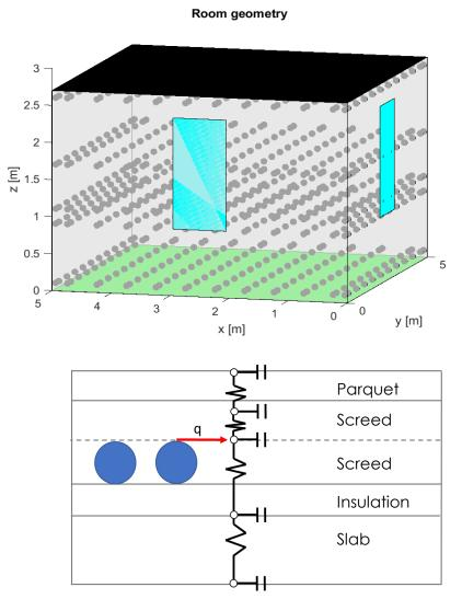
Traditional radiant floor heating (high inertia)
