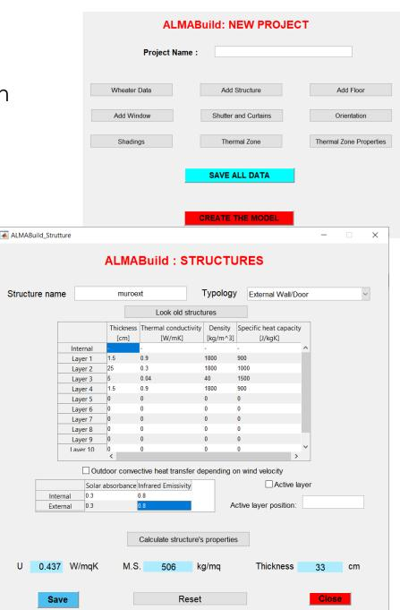
**Tool** operating in the Simulink (MATLAB) environment for the simulation of coupled **building-HVAC systems** under dynamic operating conditions.
