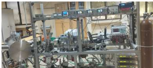
The complete energy selective high resolution 14pole RF Ion trap Time of flight mass spectrometer at AMP Lab, IIST
