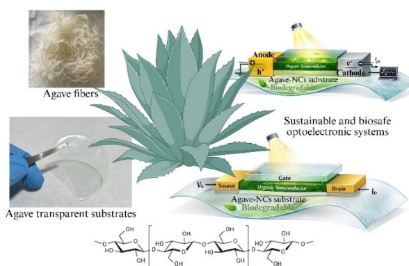
Figure 1: Conceptual schematics of sustainable and biosafe optoelectrical systems based on Agave-NCs substrates.
