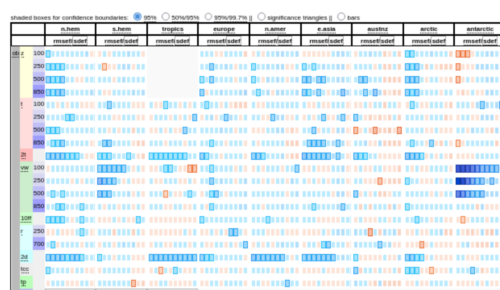
Figure 4. Scorecard vs observations for Dec 2021 – Feb 2022 and Jun-Aug 2022 combined, blue improved, orange worse. Changes in rms fit for days 1-10 shown in a row.
