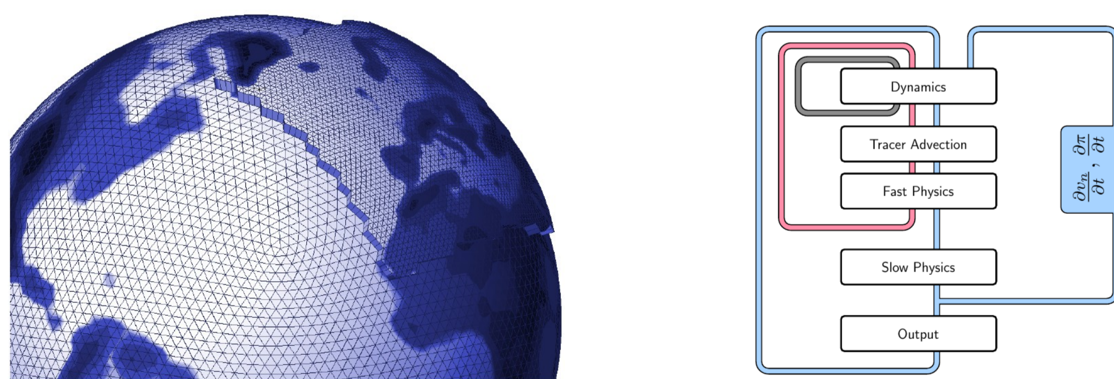
Figure 2: Left: Representation of the icosahedral grid of ICON (from the ICON tutorial) Right: Flowchart of the model structure of ICON (from the ICON tutorial)
